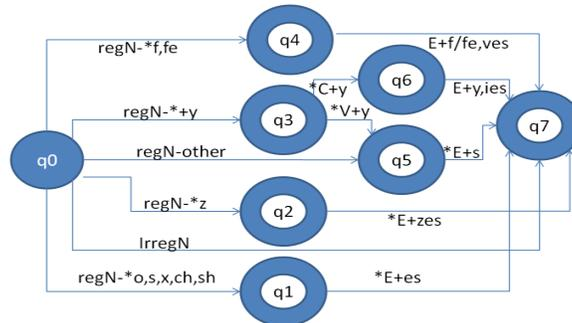
Fig. 3. Finite state automata for Singular noun to plural form.
