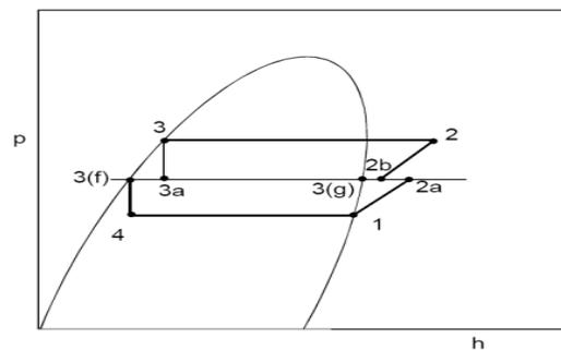
Fig. 21. Cycle of multiple compressions using flash chamber.
