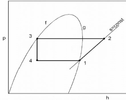
Fig. 14. Refrigeration cycle.
