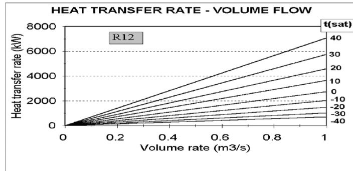
Fig. 5. Heat transfer rate versus volume rate.
