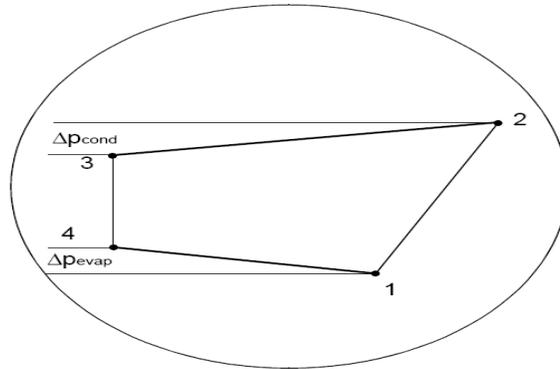
Fig. 18. Pressure drops in evaporator and condenser.
