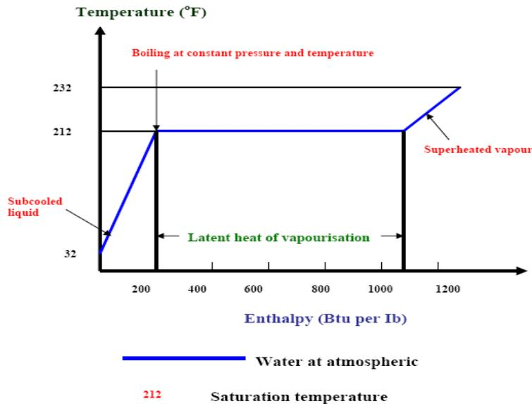
Fig. 13. Water undergoing a change of state.
