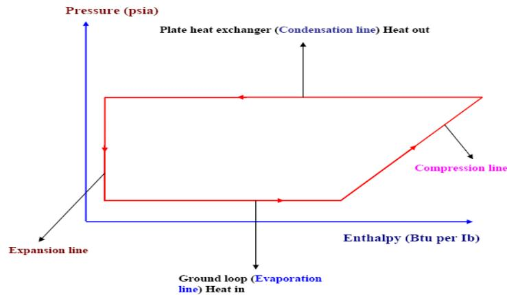
Fig. 12. The ideal cycle on Pressure-Enthalpy diagram.
