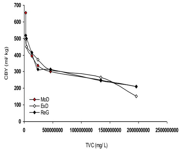
**Fig 5.** Graph of cumulative biogas yield against COD. **Fig. 6.** Graph of cumulative biogas yield against TVC.
