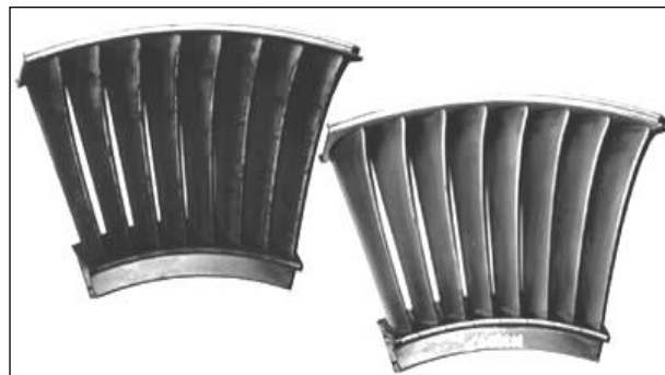
Fig. 7. Comparison of gas turbine blades in two types of filtration (Carter, 2005).
