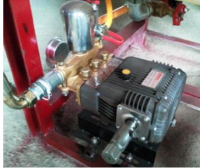
Fig. 3. Water pump and main valves.
