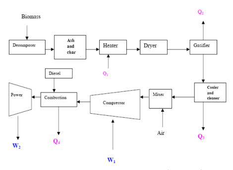
Fig. 7. Advanced biomass power with diesel engine (Omer, 2006).
