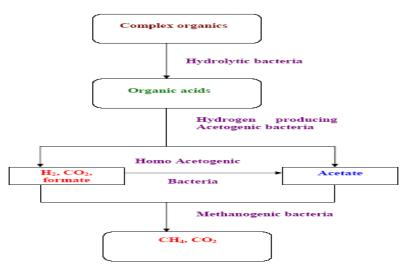
Fig. 3. Biogas production process (Omer, 2003).
