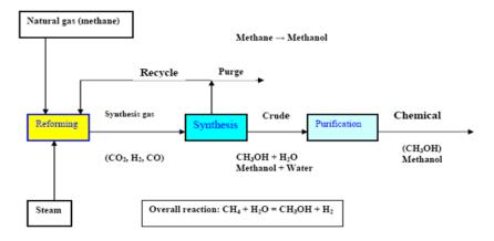
Fig. 2. Schematic diagram shows methanol production (Omer, 2006).
