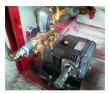
Fig. 3. Water pomp and main valves.
