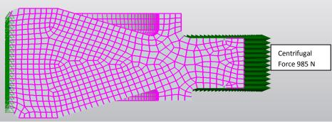
Fig. 5. Boundary conditions in structural/stress analysis.
