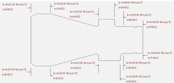
Fig. 4. Boundary conditions for thermal analysis.
