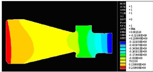
Fig. 8. Thermal stress profile along radial direction of turbine wheel.
