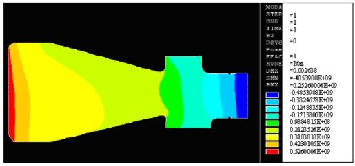
Fig. 10. Combined stress profile along disc radial direction
