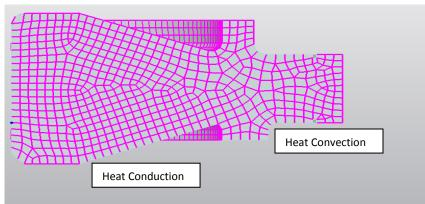
Fig. 6. Boundary conditions in thermal/heat transfer analysis.
