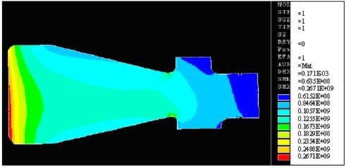
Fig. 9. Centrifugal tensile stress profile along wheel radial direction.
