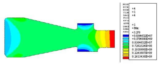
Fig. 11. Combined stress profile with residual stresses induced along disc radial direction (with hot spinning process).
