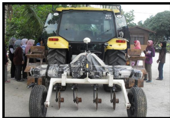
Fig. 2. The System components of veris soil EC mapping-model: Veris3100.
