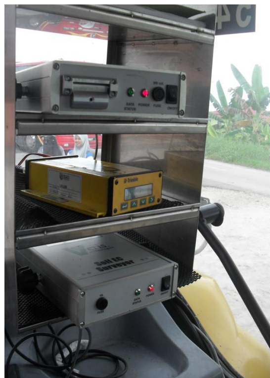
Fig. 4. Complete component of receiver that receive data from GPS and Veris Soil EC controller.
