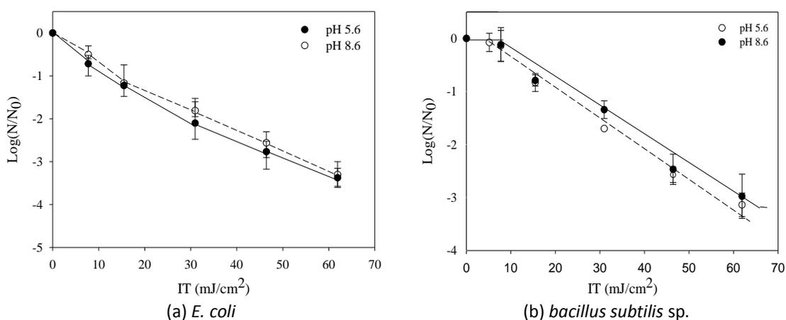
**Fig. 2.** Inactivation response of *E. coli* and *bacillus subtilis* sp. in deionized water for 260 nm UV LEDs (pH 5.6 and 8.6).
