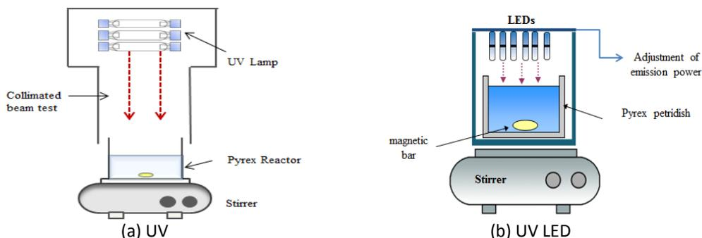
Fig. 1. Experimental equipment.
