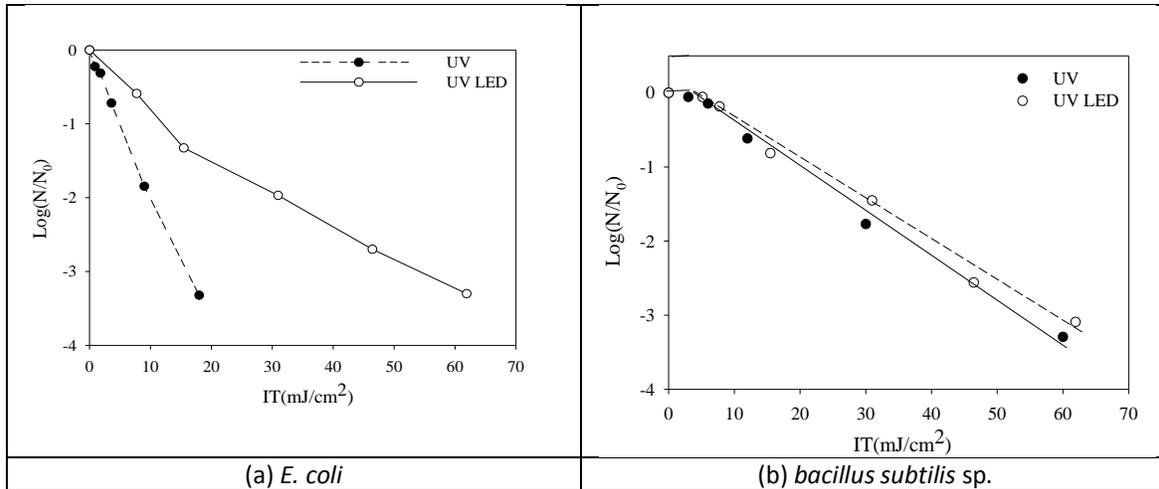
Fig. 3. Inactivation response of *E. coli* and *bacillus subtilis* sp. in deionised water for by UV and UV LEDs (pH 7).
